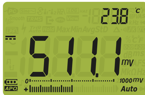
Figure 2-4 DC voltage display
