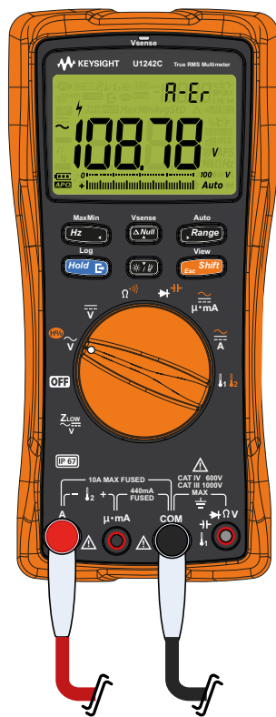
Figure 1-2 Example of wrong terminal input
